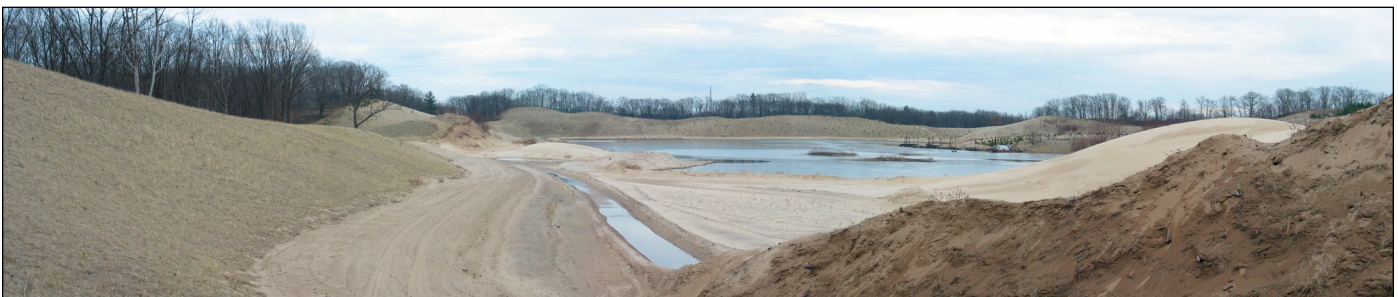
Nadeau Pit. The dredge lake continues to be expanded as sand is removed from below the water table. A 5 year extension of the permit was issued last year.
